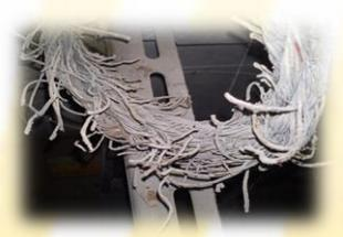
**Thorough examination** and discard criteria: A thorough examination is a visual check, performed by an expert and, when required, complemented with other methods, e.g. measurement and/or tests with intent to identify any damage or deterioration that might affect the slings fitness for use.
